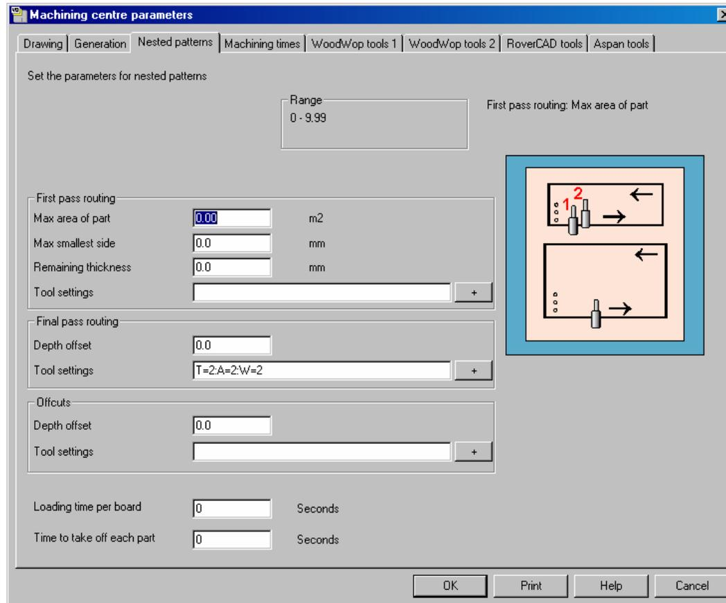
Figure 7-26 Machining centre parameters (Nesting)
