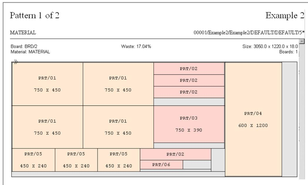
Figure 6-01 Pattern - recuts and head cuts
